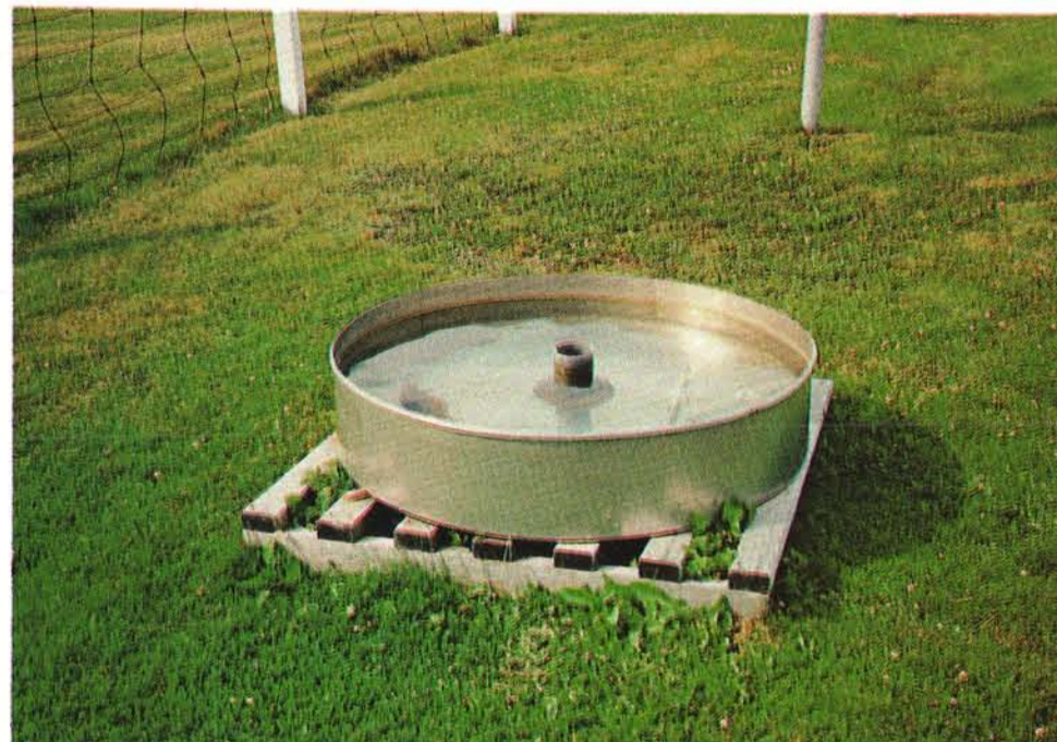
Figure 10.1 Class A Evaporation Pan
