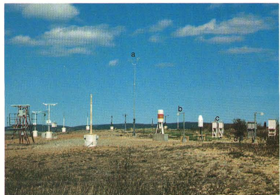
Figure 5.1 Weather Station at St. John's Airport (a) Anemometer (Wind speed and direction) (b) Snow Depth Sensor (c) Stevenson Screen (Thermometers) (d) Tipping Bucket Rain gauge
