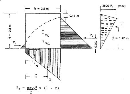
min contact area would be small, probably governed by crushing strength of ice in the limit. Conservatively (1 - r) = 1
