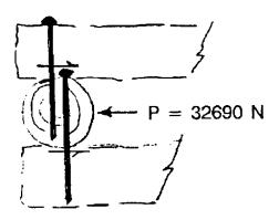
Garfinkel (1973) page 173 suggests that the actual factor of safety for the recommended load on a nailed connector  $\approx$  6.0.
